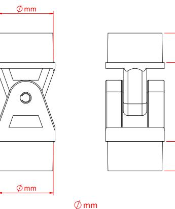
Ømm T58730 - 47mm T58731 - 44mm T58733 - 41.5mm T58734 - 39.5mm
